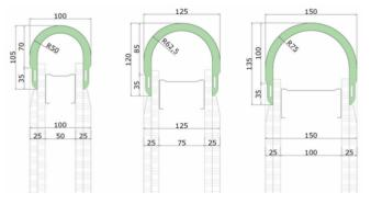
The Gyrex curved U-profile is available in various wall thicknesses, each with a length of 3000 mm.
